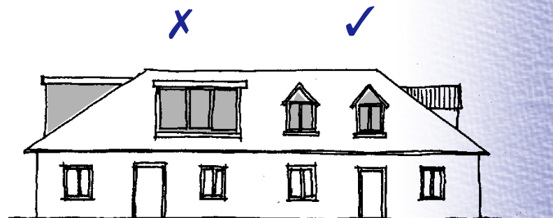
Dormer windows should match the house
