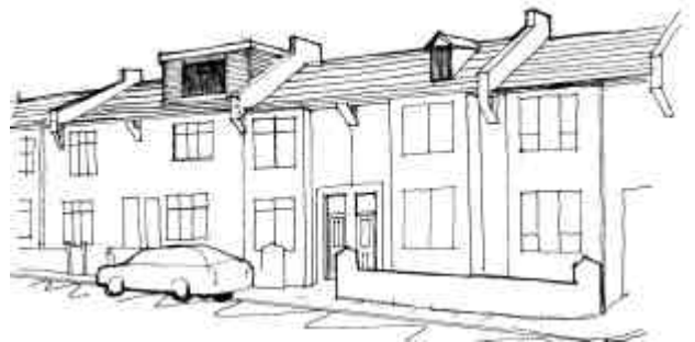
A uniform terrace disrupted by dormers
