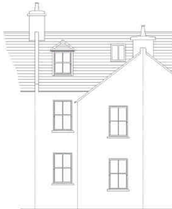
A well proportioned and positioned dormer and rooflight
