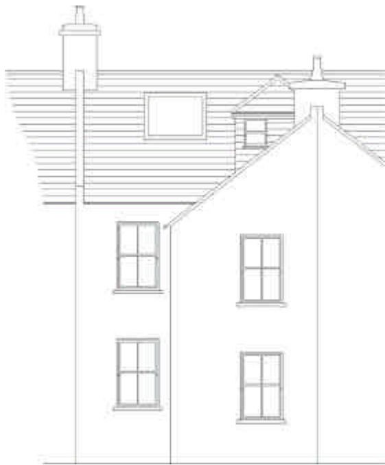
A poorly proportioned and positioned dormer and rooflight
